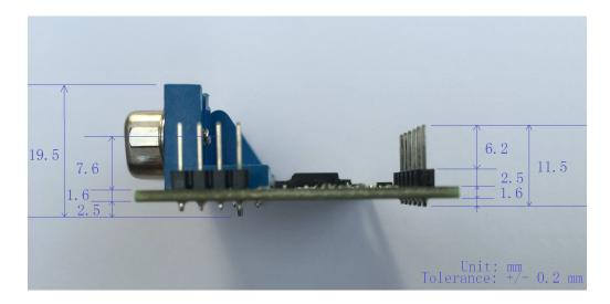
Fig. 2 GPIB to UART Module Mechanic Size (side view)
