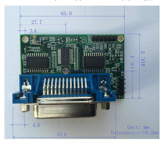
Fig. 1 GPIB to UART Module Mechanic Size (top view)
